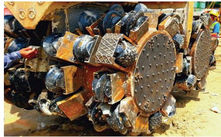
Roller cutters to diaphragm wall
