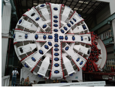
TBM Cutting Head ( Note )
