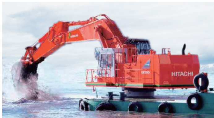
On barge excavator of 180-tonne class
