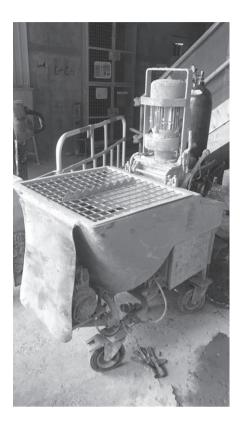
A plaster spraying machine is a type of machine which enables a plasterer to skim a wall more quickly than using a hand float manually. The main benefit of using a plaster spraying machine is to speed up the plastering process. For wet trades projects involving plastering works, we have increasingly used plaster spraying machines to replace manual operation so as to lower labour costs and further enhance our craftsmanship.
