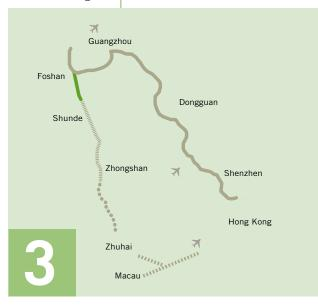
he Phase I West is a 14.7 km closed system dual three-lane expressway. It connects to the ESW Ring Road in the north and to the National Highway 105 and Bigui Road of Shunde in the south.
