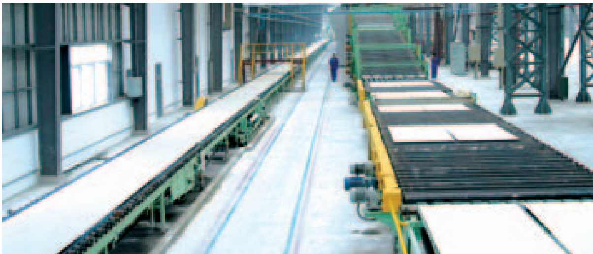
Taicang gypsum board production line of BNBM commenced operation on 5 November 2008 with an annual capacity of 30 million square metres.
