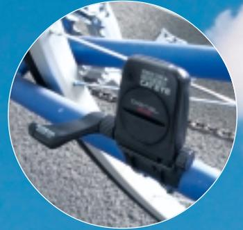
Award-winning cycling computer which monitors user's heart rate, cycling speed, cadence, etc. via a 2.4GHz wireless digital transmission.
