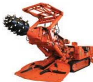
EBZ200A roadheader, with a cutting power of 200kw.
