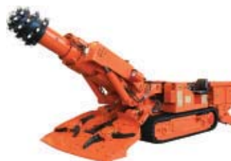
EBZ135 roadheader, with a cutting power of 135kw.
