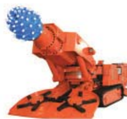
EBZ260 roadheader, with a cutting power of 260kw.
