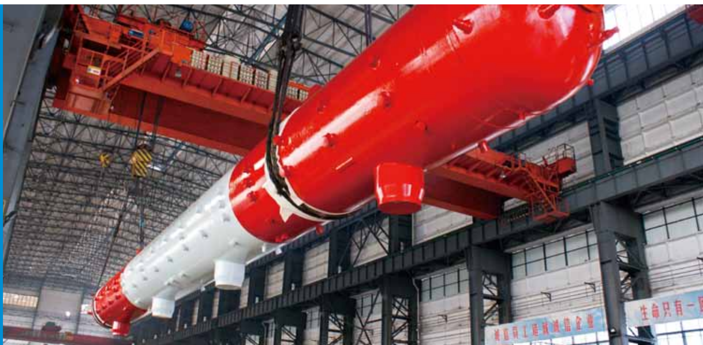
Power station boiler steam drum
