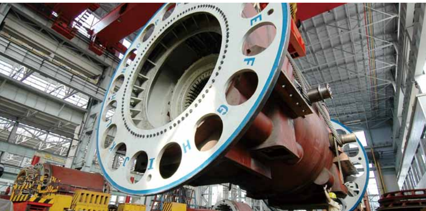
60MW steam turbine generators unsplit frame
