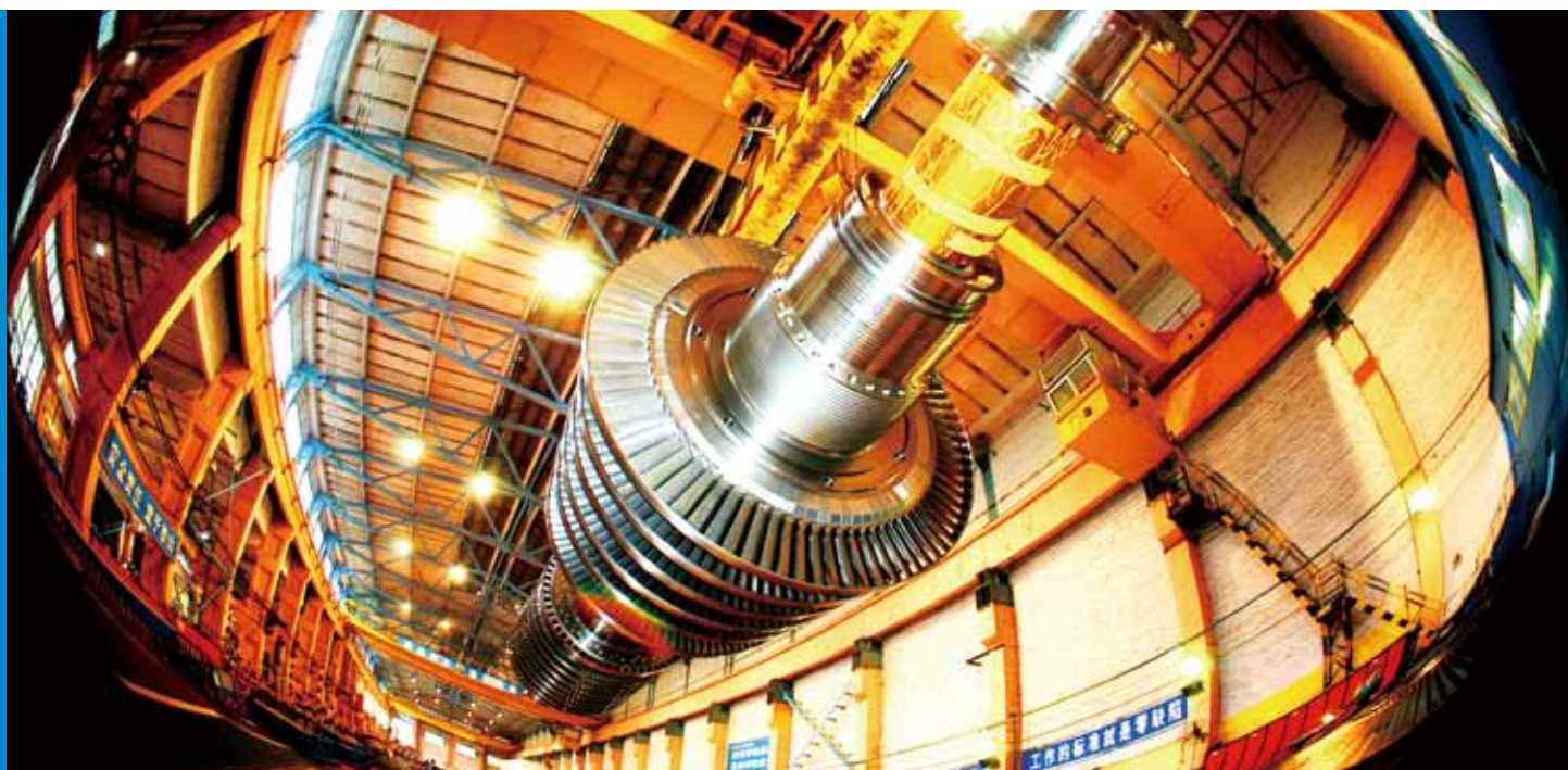
Steam turbine rotor
