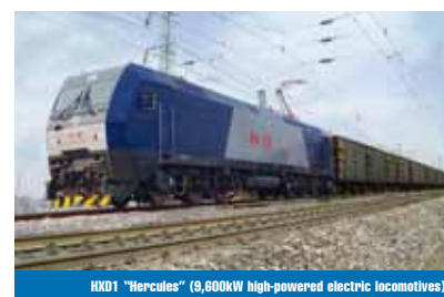
HXD1 "Hercules" (9,600kW high-powered electric locomotives)
