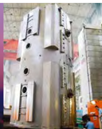
Stator frame of nuclear power generator
