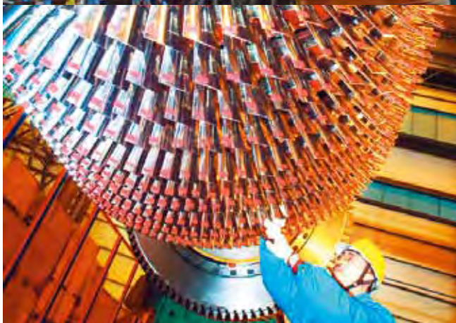
Rotor of gas turbine
