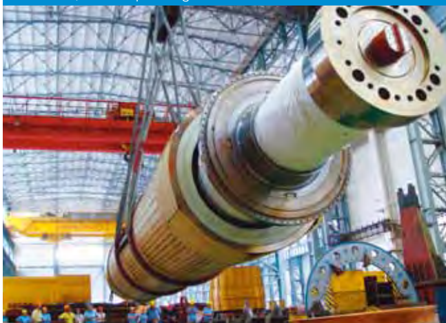
Rotor of 1,000MW power generator
