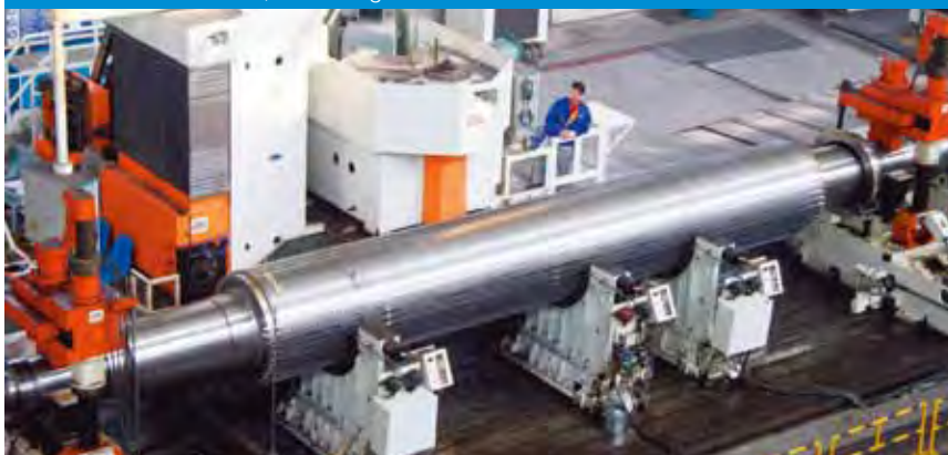
Production of rotor of 1,000 MW generator
