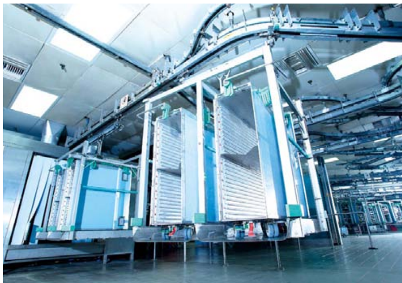
Cathay Pacific Catering Services uses gas-powered steam washers and dryers to clean and dry the utensils, meal carts and meal trays used on flights.
