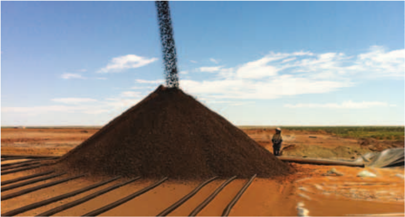
Figure 5: Stacking commences for the first transition production trial
