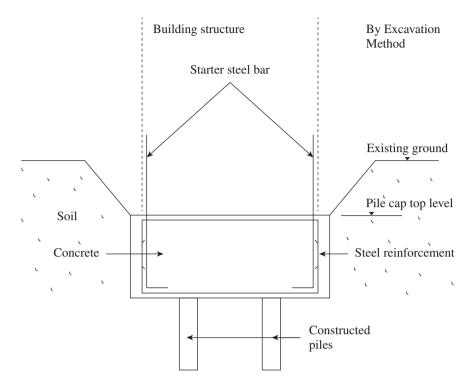
Pile caps are concrete structures built on the head of a pile or a group of piles for transmission of loads from the structure above to the pile or group of piles.
