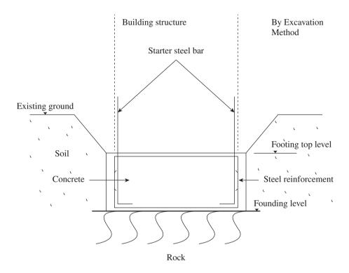
Footing foundation is a type of shallow foundation which transfers building loads to a shallow bedrock layer which is near the ground surface, usually less than two meters below ground. Most of the footings are formed by concrete poured into a trench and constrained by some kind of forms. Functionally, footings are similar to pile caps. However, footings transfer the load directly to the bedrock while pile caps transfer the load onto piles.
