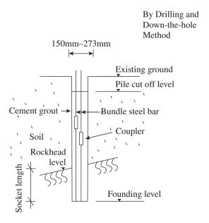
A mini-pile usually consists of one or more steel bars encased by grout inside a drill hole not exceeding 400 mm in diameter. They are normally designed to be socketed into rock and are mainly used to resist compression or tension loads on sites with difficult access. Steel casing are to be provided to support the pre-drilled hole within the soil and/or fractured rock during drilling operation.
