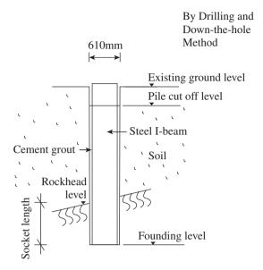
Socketed H-piles (also known as pre-bored H-piles) are installed by inserting prefabricated steel H-piles into pre-bored holes (typically about 550 mm in diameter) sunk into bedrock, and subsequently grouting the holes with cementitious materials.
