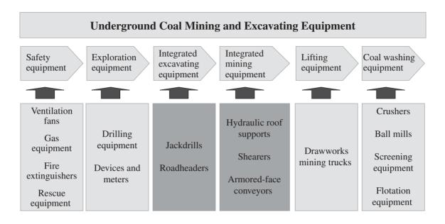
In normal industry terms and in the context of this prospectus, coal mining and excavating equipment typically refers to hydraulic roof supports, shearers, armored-face conveyors and roadheaders which, together, are also known as "Three Machines and One Roof Support."
