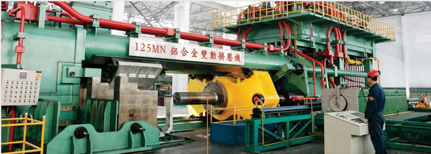
The Group is equipped with a range of advanced large-scale extrusion production lines, with core equipment imported mainly from Europe. These facilities enable the Company to produce large-section, high quality, high value-added aluminium extrusion products on a large scale.
