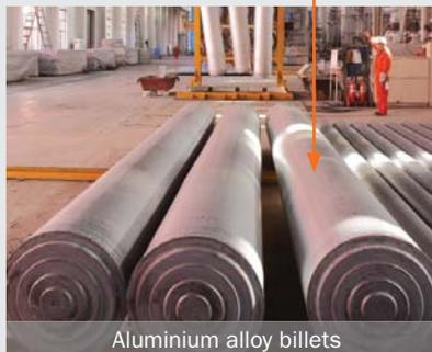
The Group owns and operates industry leading aluminium smelting and casting facilities, with LPG-powered tilt smelting furnaces. These facilities enable the Group to apply customized alloy formulae to produce aluminium alloy billets to meet different needs. Such facilities and technical knowhow are prerequisites for producing high-end industrial aluminium extrusion products.
