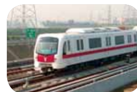
Linear motor driving metro vehicle
