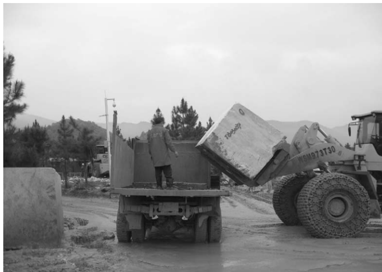
Figure 8.15. Loading block onto a truck for shipment
