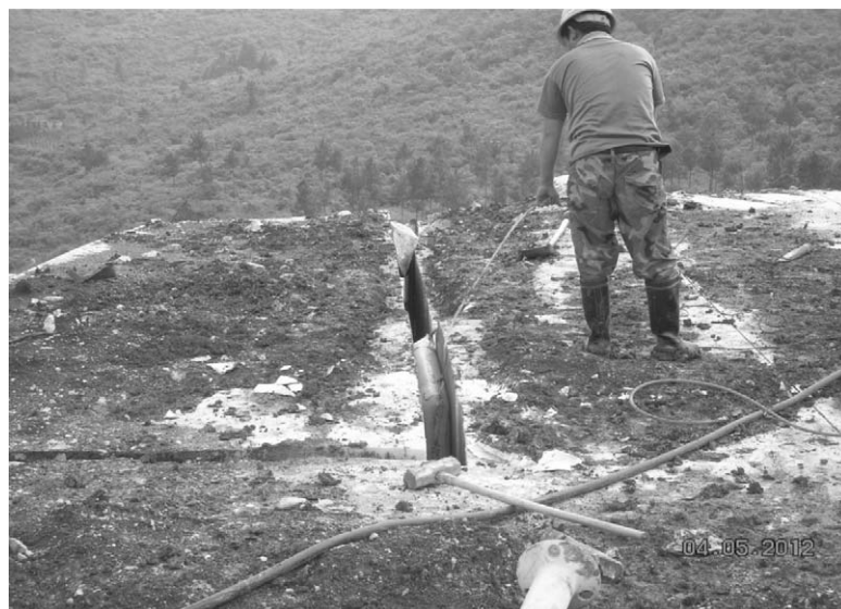
Figure 8.9. Set inflation air bag for large rectangular stone overturning
