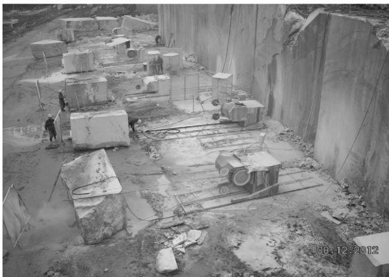
Figure 8.13. Block trimming after separation
