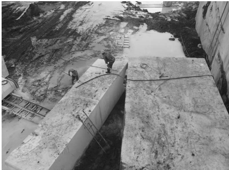
Figure 8.12. Separation of overturned large rectangular stone into smaller commercial blocks
