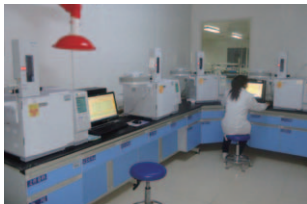
氣相色譜：三聚氰胺檢測 Gas chromatography: melamine inspection
