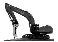
A breaker is a powerful percussion hammer fitted to an excavator for demolition, construction and quarrying. It is powered by an auxiliary hydraulic system from the excavator which is fitted with a foot-operated valve for this purpose.
