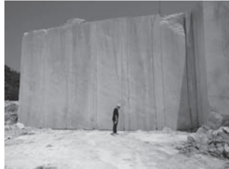
Quarry face is cut by both horizontal and vertical diamond belt saws.
