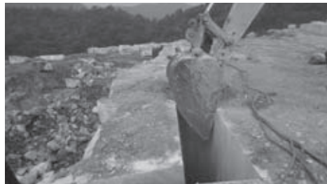
Tilting down of rectangular primary blocks by a front end-loader.
