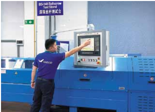
A HAECO Component Overhaul (Xiamen) technician conducts a receiving inspection of a Boeing 737NG flap ballscrew on the OEM test stand.
