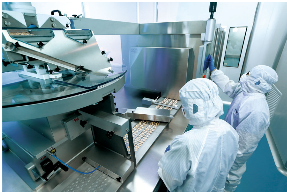
High precision automated tablet and capsule blister machine
