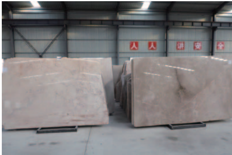
Figure 10-1: Polished slabs of Carlo Rose (left) and Royal Beige processed by the Processing Plant
