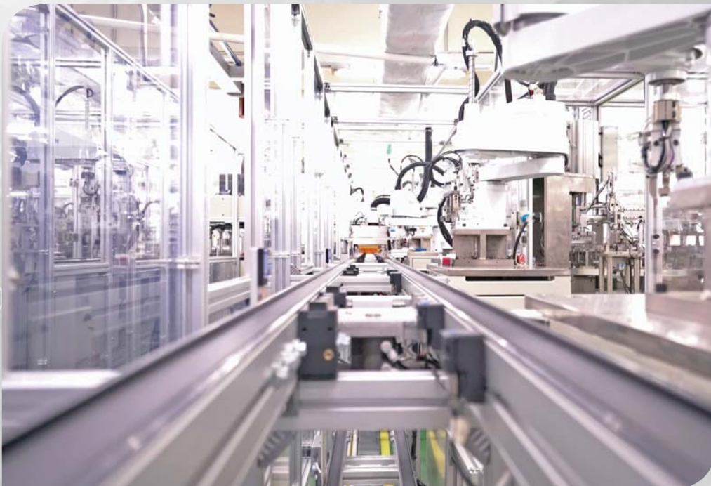
Fully automated assembly line for dishwasher drain pumps.
