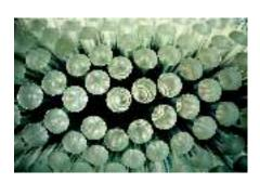
Ceramic ferrules are currently regarded as the best type of connector compared to plastic, stainless steel and aluminium connectors since ceramic ferrules are durable, environmentally stable, and easy to bond with optical fiber. They also have the highest degree of precision in the transmission of optical signals and can closely match the degree of expansion and contraction of optical fibers as a result of temperature change.
