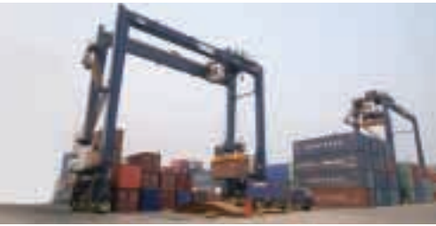
Rubber Tyred Gantry Crane
