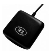
The ACR39 is the successor of the Group's very successful ACR38U product line and acts as a new generation PC-linked reader with a higher speed. ACR39 has improved features such as a higher speed in operation and has programmable software capability (i.e. upgrading the firmware in a simple process by using a PC rather than by resorting to the cumbersome work in the factory), serial interface on top of USB interface, etc.
