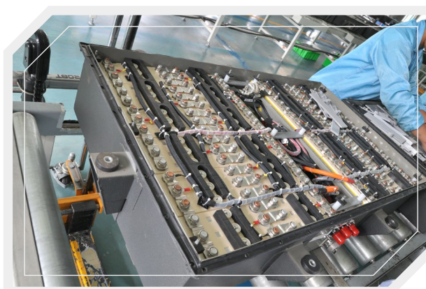
Sophisticated integration and combination of battery pack battery cells into a battery pack
