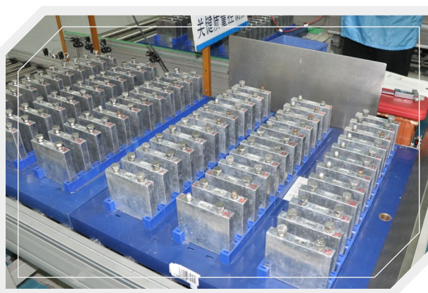
Checking and quality control on battery cells
