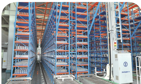
Batteries stored systematically pending the next production process
