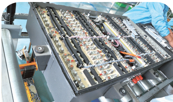
Sophisticated integration and combination of battery pack battery cells into a battery pack
