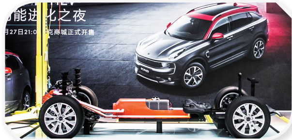
Lynk 01 PHEV battery pack produced by Zhejiang Forever New Energy
