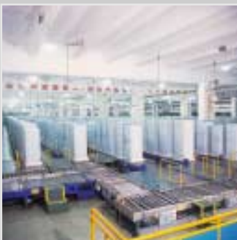
Twenty-four-hour refrigeration testing lines for refrigerator production
