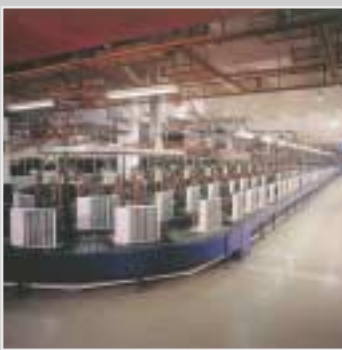
Testing lines for air-conditioner production
