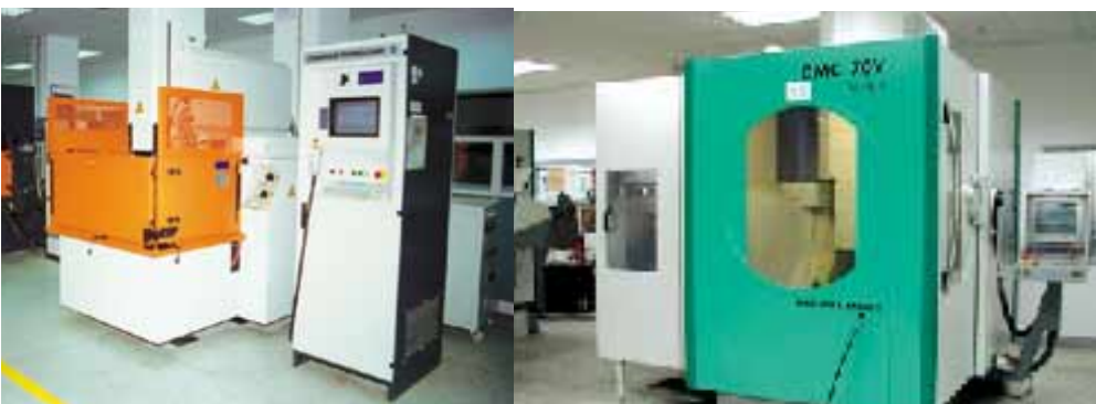
(left to right) Electrical Discharge machine, Computer Numeric Control (CNC) machine centre
