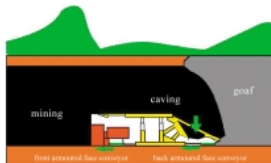
Long-wall top coal caving technology
