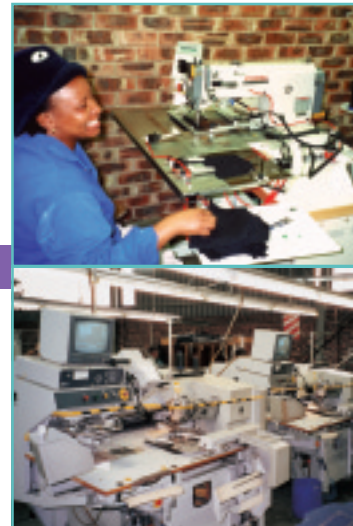
Supreme Bright Group Limited equips with modernized production facilities including back pocket fancy stitching machine (Top) and automatic patch pocket machines (Bottom).
