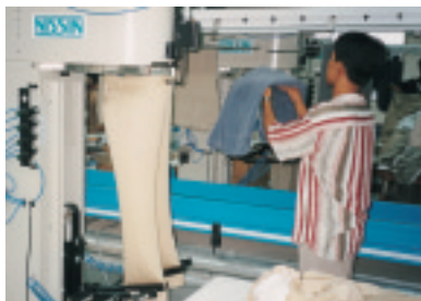
PT Aneka, a woven bottom factory in Indonesia, equips with trousers finisher machines.
