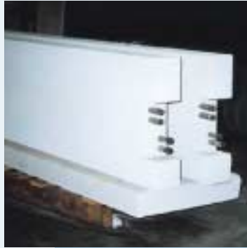
Conduits embedded into panel
