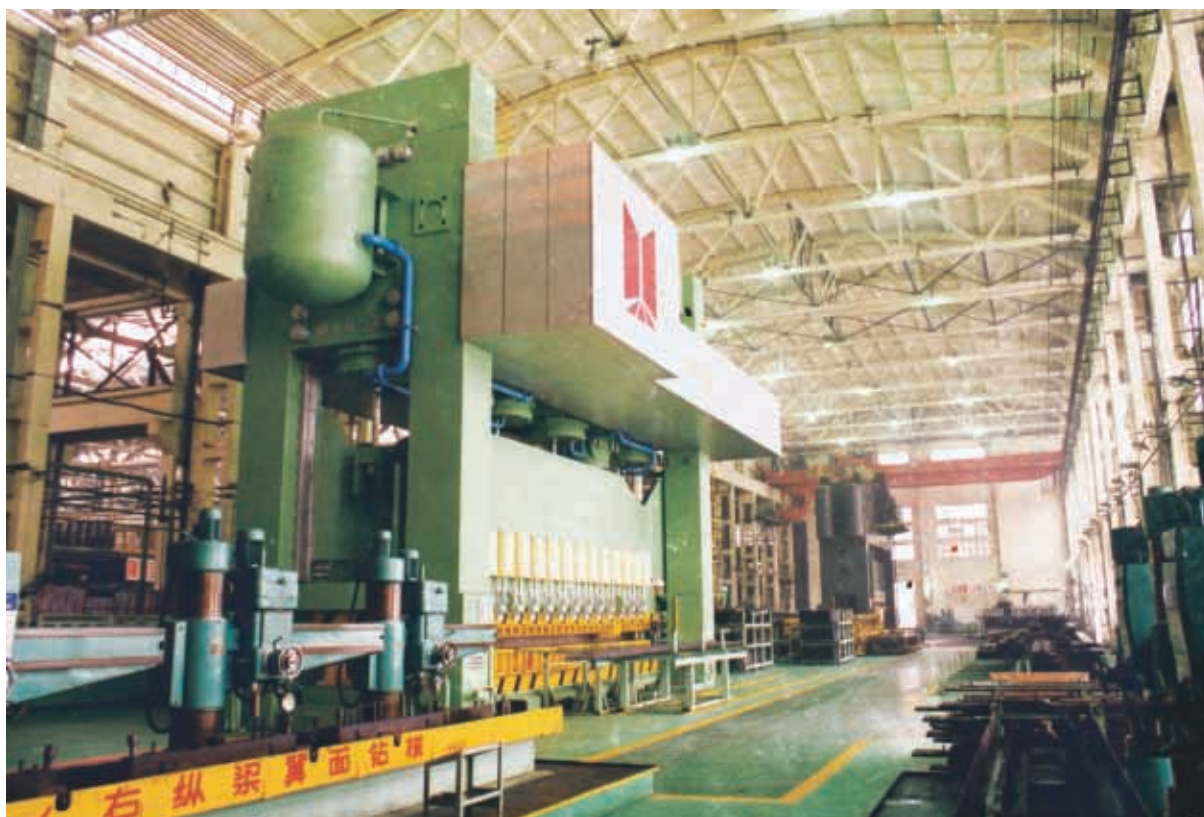
國內最大5,000噸機械壓機 The biggest 5,000 tons mechanical pressing machine in China
