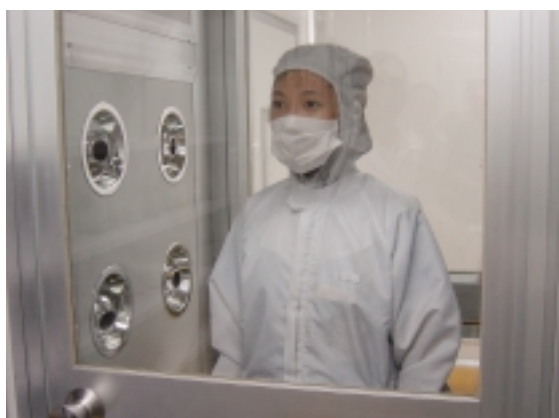
進入無塵車間前必需經氣流室除塵 Passing through Air-Shower for removing dust before entering Clean-Room
