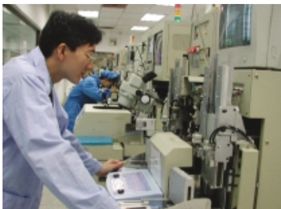
調整全自動晶體管裝配設備 Setting up of fully automatic bonders for transistor assembly
