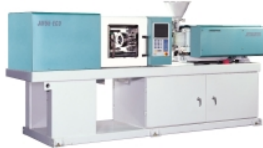
全電式注塑機 JM55-ECO JM55-ECO All-electric Injection Moulding Machine
