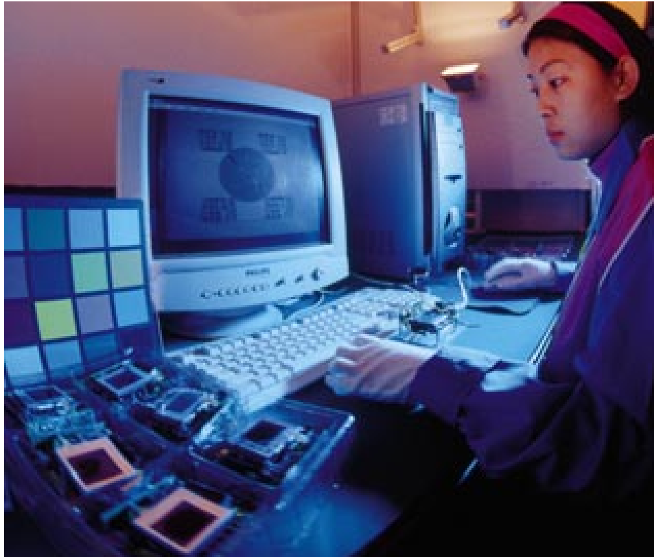
A Hutchison Harbour Ring operator is tuning the focus of an optical lens on a CMOS sensor – a critical process in making a quality digital camera.
