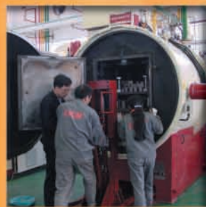
Loading and Unloading of a Vacuum Furnace 真空熱處理爐裝卸情況
