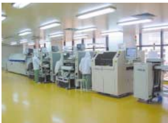
電子專業生產用之貼片設備 Surface Mounted Facilities for EMS Projects
