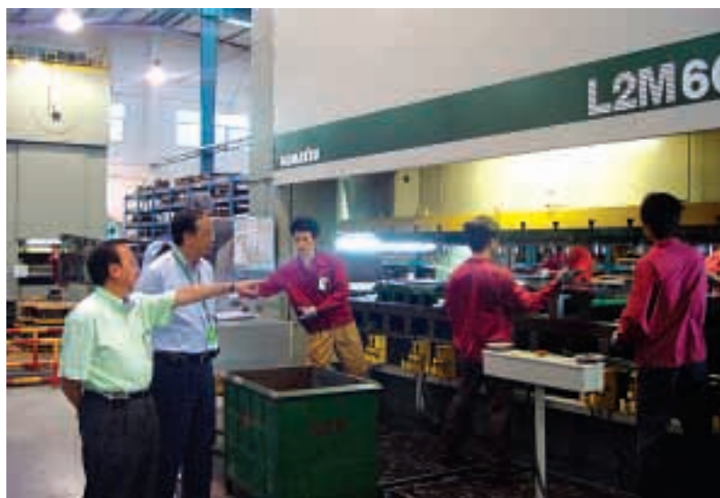
Money well-spent: The new 600-tons metal stamping machine facilitating the introduction of progressive stamping die.
