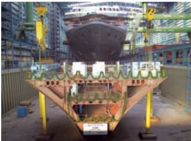
The first of 67 keel blocks that will complete the hull of NCL America's Pride of Hawaii. In the background is NCL Corporation's Norwegian Jewel, scheduled for delivery in August 2005.
