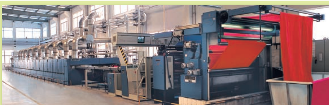
Monfongs 328/329 TwinAir Stenter Frame Range
