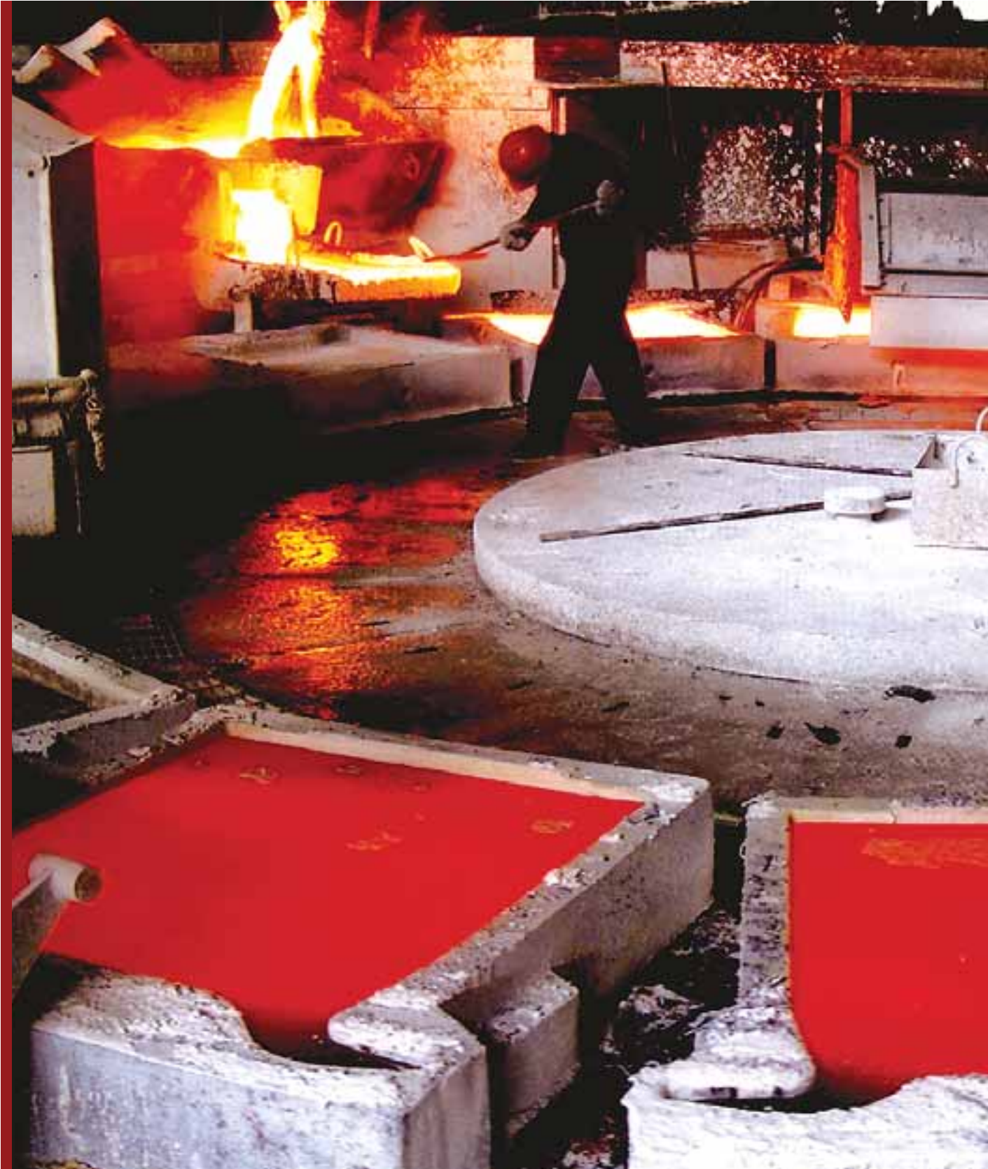
Anode casting machine in Qingyuan smelting plant
