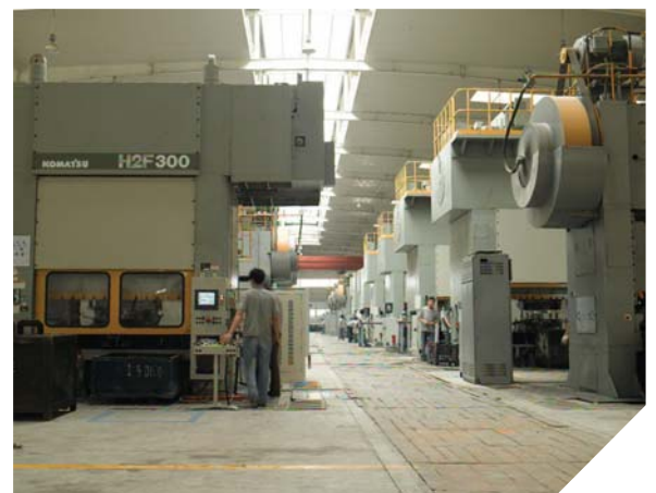
Stamping machines for steel backings
