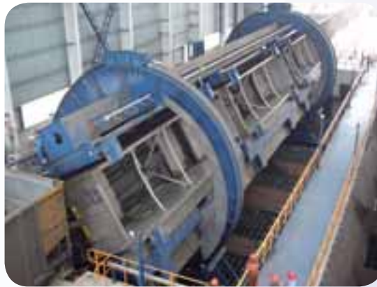
The triple unloading system developed and manufactured by ZPMC
