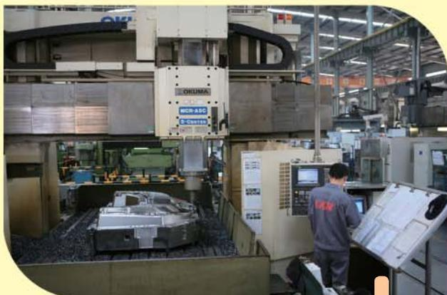
Production of mould base for the instrument panel of an automobile needs stock of big steel block together with proper heavy-duty machines
