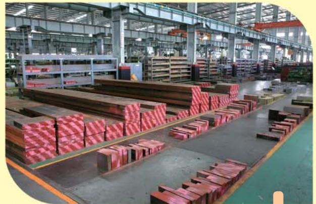
Using the colour code to distinguish different steel types systematically
