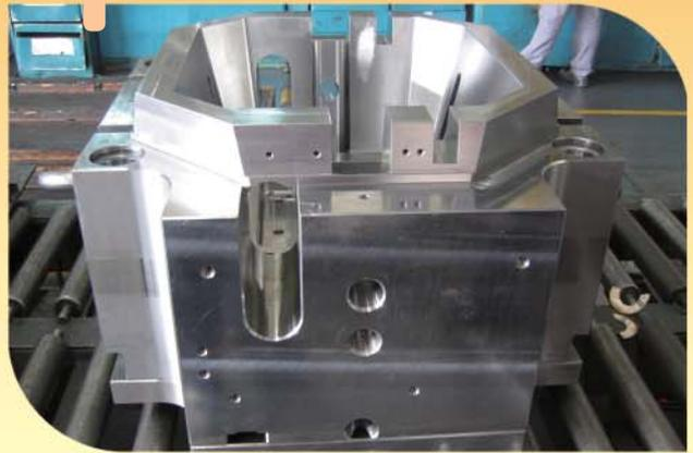
Mould base with complicated shape can be machined by using the 4th axis rotation on a horizontal machining center
