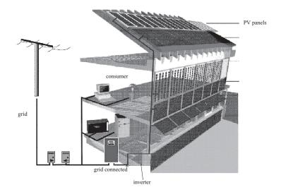
An example of a BIPV system is illustrated as follows:
